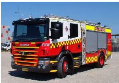
Urban pumping appliance: 15 tonnes (Gross Vehicle Mass)
