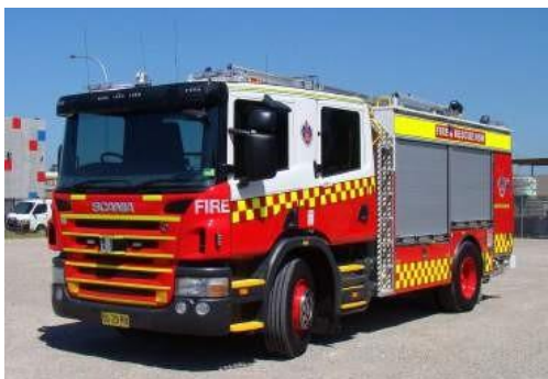
Urban pumping appliance: 15 tonnes (Gross Vehicle Mass)
