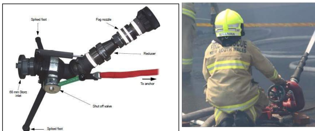
Figure 9 A firefighting monitor
