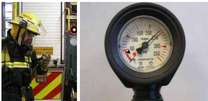
Figure 31 Self contained breathing apparatus pressure gauge
