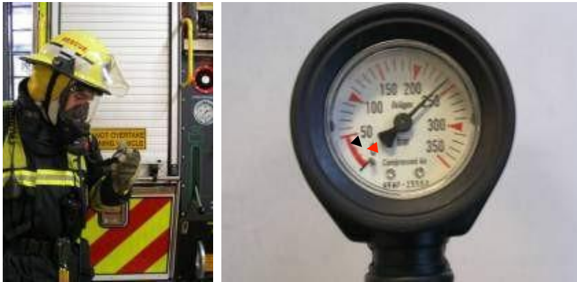
Figure 31 Self contained breathing apparatus pressure gauge
